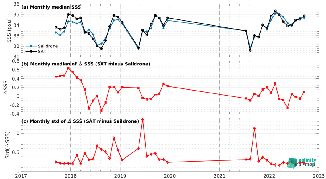
Figure 8: Time series of the monthly median SSS (top), median of \Delta\text{SSS} (Satellite - Saildrone) and Std of \Delta\text{SSS} (Satellite - Saildrone) over the Pacific Ocean Pi-MEP region considering all match-ups collected by the Pi-MEP.
