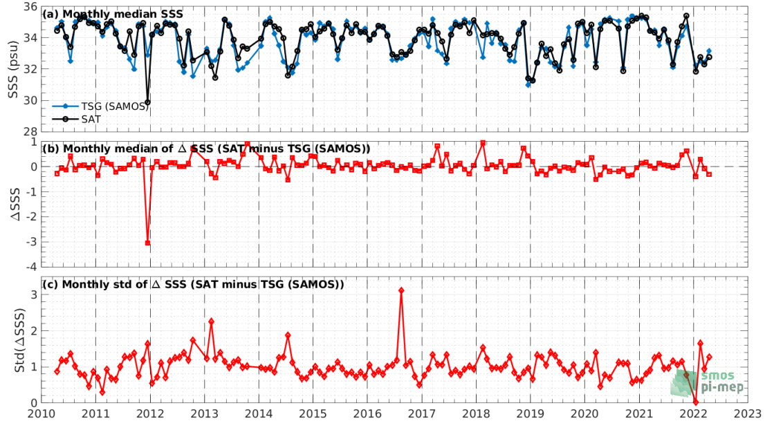
Figure 7: Time series of the monthly median SSS (top), median of \Delta SSS (Satellite - TSG (SAMOS)) and Std of \Delta SSS (Satellite - TSG (SAMOS)) over the Pacific Ocean Pi-MEP region considering all match-ups collected by the Pi-MEP.
