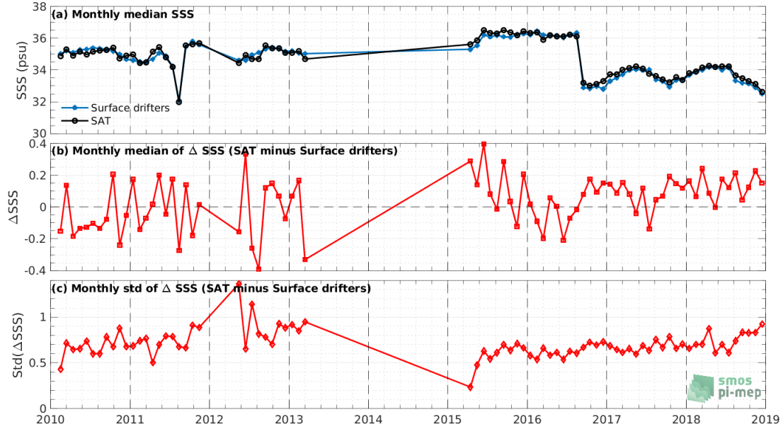
Figure 6: Time series of the monthly median SSS (top), median of \Delta SSS (Satellite - Surface drifters) and Std of \Delta SSS (Satellite - Surface drifters) over the Pacific Ocean Pi-MEP region considering all match-ups collected by the Pi-MEP.
