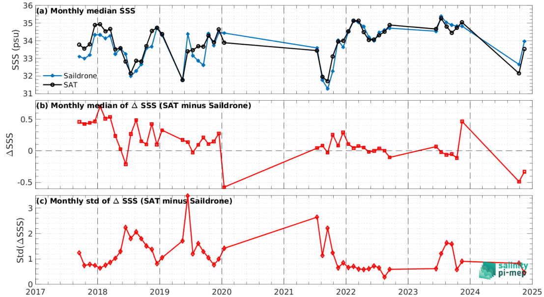
Figure 8: Time series of the monthly median SSS (top), median of \Delta\text{SSS} (Satellite - Sairdrone) and Std of \Delta\text{SSS} (Satellite - Sairdrone) over the Pacific Ocean Pi-MEP region considering all match-ups collected by the Pi-MEP.
