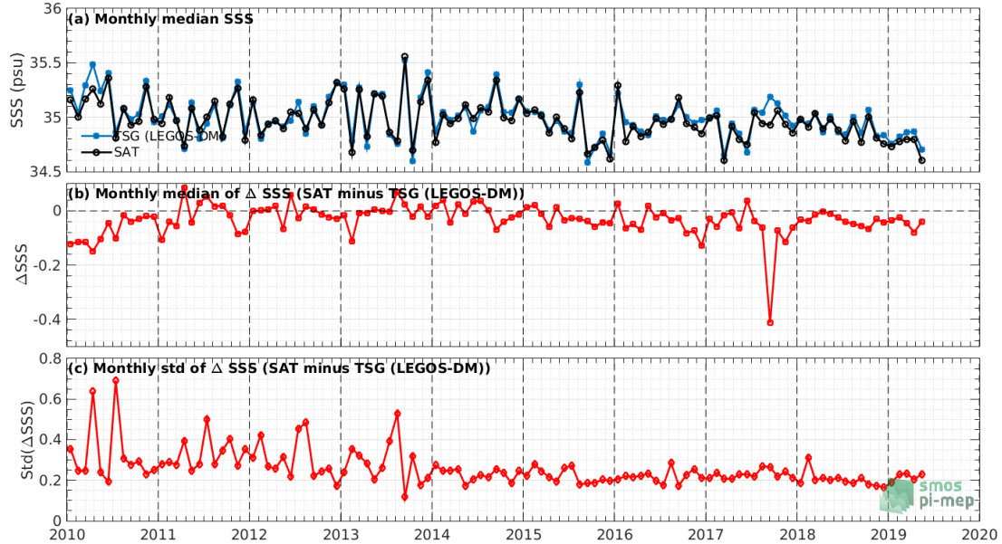
Figure 7: Time series of the monthly median SSS (top), median of \Delta\text{SSS} (Satellite - TSG (LEGOS-DM)) and Std of \Delta\text{SSS} (Satellite - TSG (LEGOS-DM)) over the Pacific Ocean Pi-MEP region considering all match-ups collected by the Pi-MEP.
