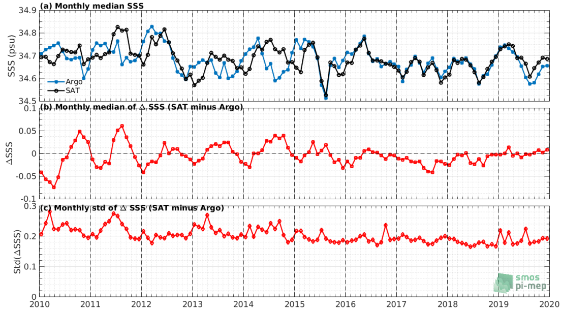
Figure 7: Time series of the monthly median SSS (top), median of \Delta\text{SSS} (Satellite - Argo) and Std of \Delta\text{SSS} (Satellite - Argo) over the Pacific Ocean Pi-MEP region considering all match-ups collected by the Pi-MEP.
