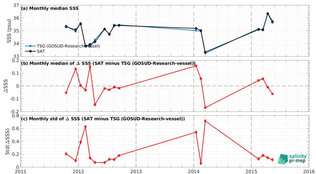
Figure 8: Time series of the monthly median SSS (top), median of \Delta SSS (Satellite - TSG (GOSUD-Research-vessel)) and Std of \Delta SSS (Satellite - TSG (GOSUD-Research-vessel)) over the Pacific Ocean Pi-MEP region considering all match-ups collected by the Pi-MEP.
