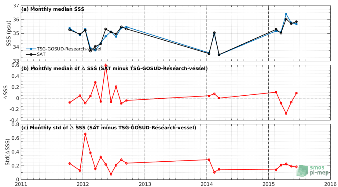
Figure 7: Time series of the monthly median SSS (top), median of \Delta SSS (Satellite - TSG-GOSUD-Research-vessel) and Std of \Delta SSS (Satellite - TSG-GOSUD-Research-vessel) over the Pacific Ocean Pi-MEP region considering all match-ups collected by the Pi-MEP.
