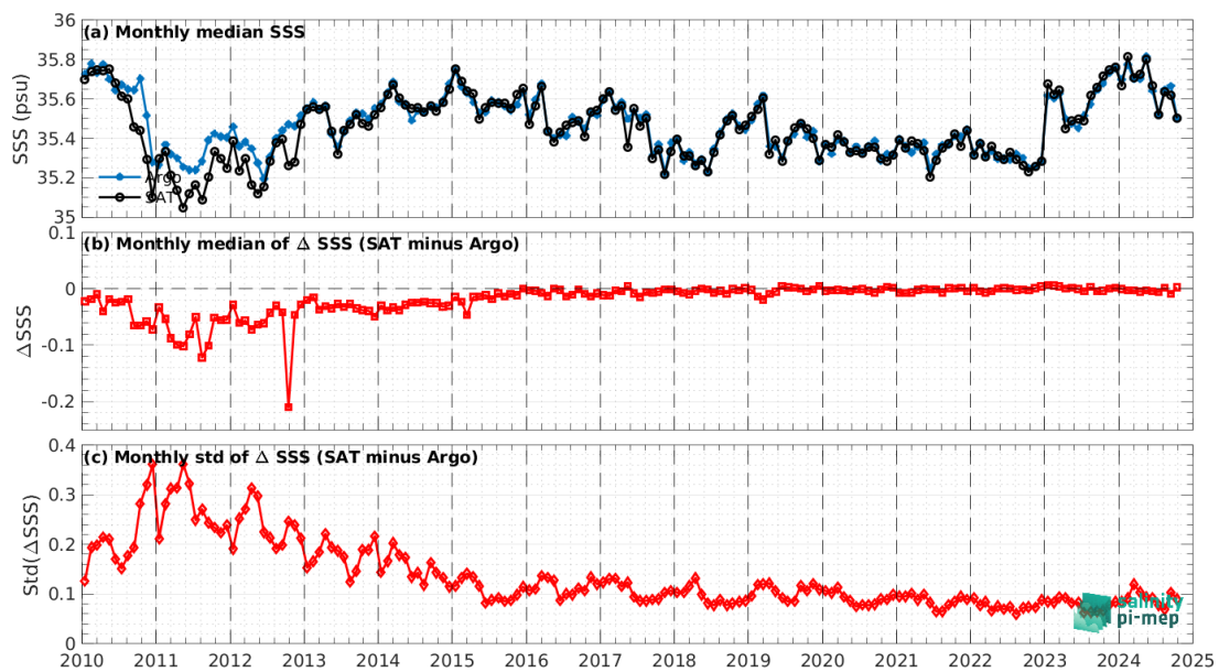
Figure 8: Time series of the monthly median SSS (top), median of \Delta SSS (Satellite - Argo) and Std of \Delta SSS (Satellite - Argo) over the OTT zone Pi-MEP region considering all match-ups collected by the Pi-MEP.
