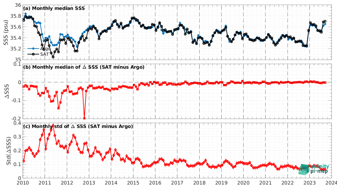
Figure 7: Time series of the monthly median SSS (top), median of \Delta SSS (Satellite - Argo) and Std of \Delta SSS (Satellite - Argo) over the OTT zone Pi-MEP region considering all match-ups collected by the Pi-MEP.
