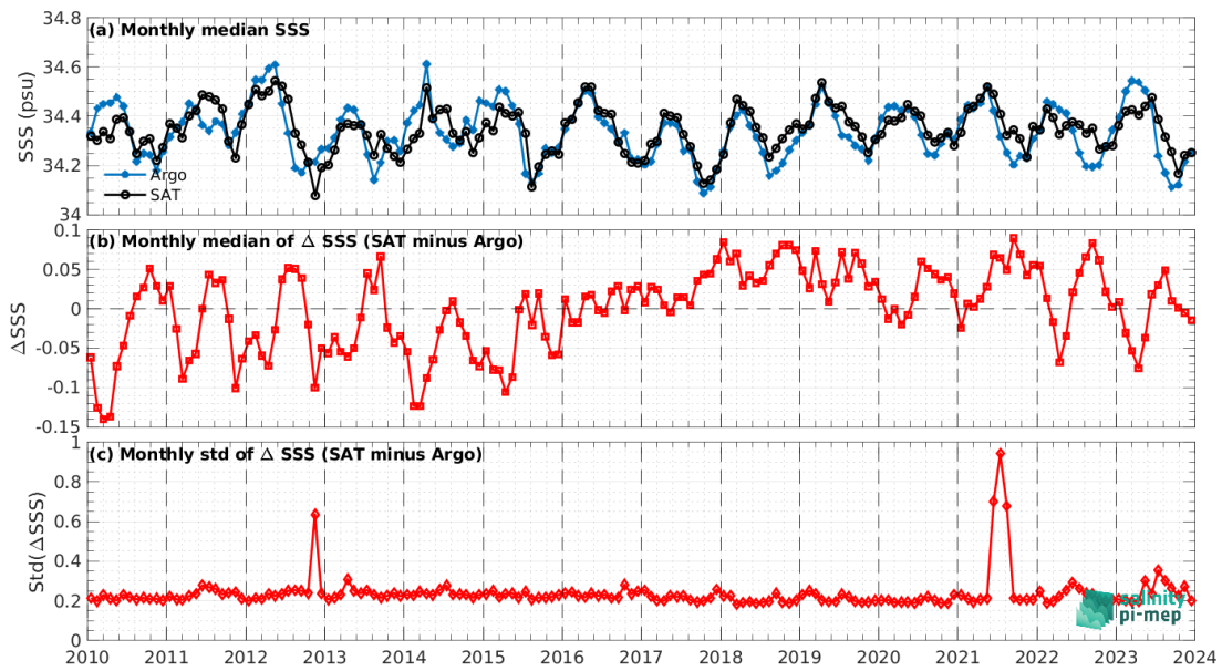
Figure 8: Time series of the monthly median SSS (top), median of \Delta SSS (Satellite - Argo) and Std of \Delta SSS (Satellite - Argo) over the North Pacific Ocean Pi-MEP region considering all match-ups collected by the Pi-MEP.
