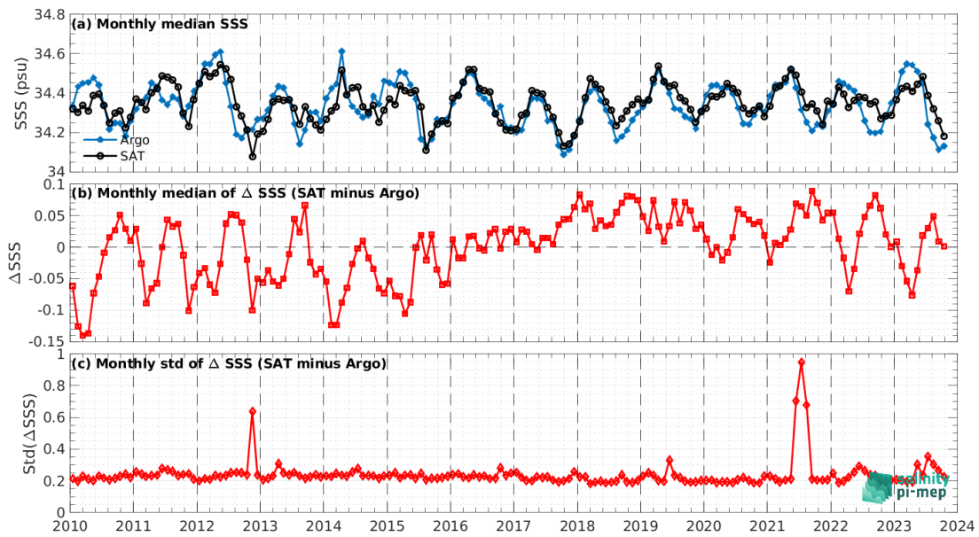
Figure 7: Time series of the monthly median SSS (top), median of \Delta SSS (Satellite - Argo) and Std of \Delta SSS (Satellite - Argo) over the North Pacific Ocean Pi-MEP region considering all match-ups collected by the Pi-MEP.
