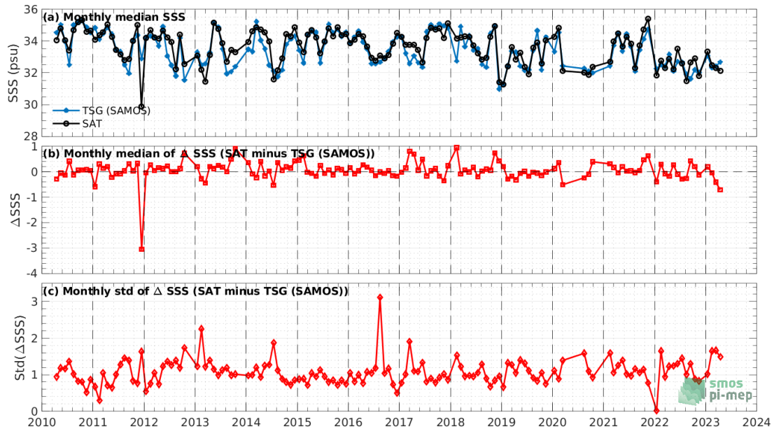
Figure 7: Time series of the monthly median SSS (top), median of \Delta SSS (Satellite - TSG (SAMOS)) and Std of \Delta SSS (Satellite - TSG (SAMOS)) over the North Pacific Ocean Pi-MEP region considering all match-ups collected by the Pi-MEP.
