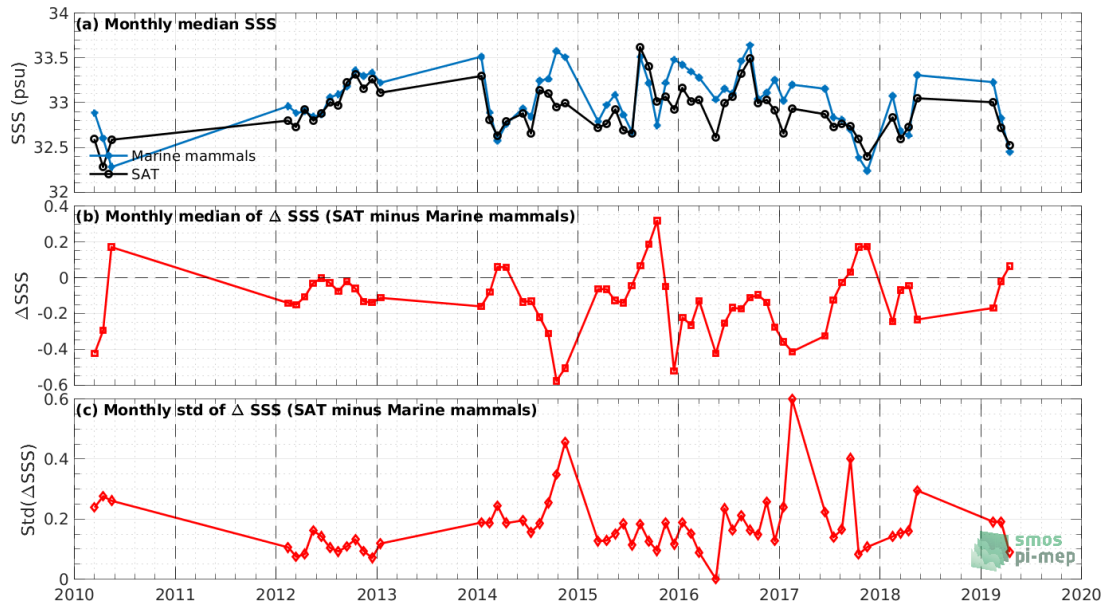
Figure 7: Time series of the monthly median SSS (top), median of \Delta SSS (Satellite - Marine mammals) and Std of \Delta SSS (Satellite - Marine mammals) over the North Pacific Ocean Pi-MEP region considering all match-ups collected by the Pi-MEP.
