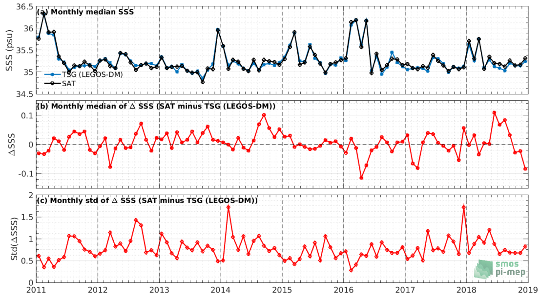
Figure 7: Time series of the monthly median SSS (top), median of \Delta SSS (Satellite - TSG (LEGOS-DM)) and Std of \Delta SSS (Satellite - TSG (LEGOS-DM)) over the North Atlantic Ocean Pi-MEP region considering all match-ups collected by the Pi-MEP.
