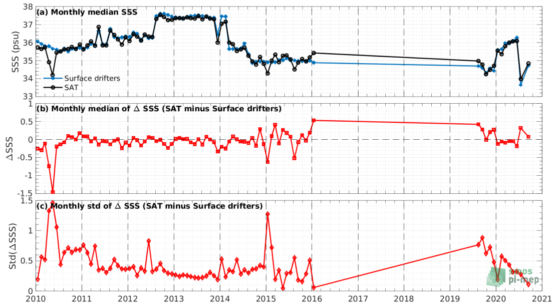
Figure 6: Time series of the monthly median SSS (top), median of \Delta SSS (Satellite - Surface drifters) and Std of \Delta SSS (Satellite - Surface drifters) over the North Atlantic Ocean Pi-MEP region considering all match-ups collected by the Pi-MEP.
