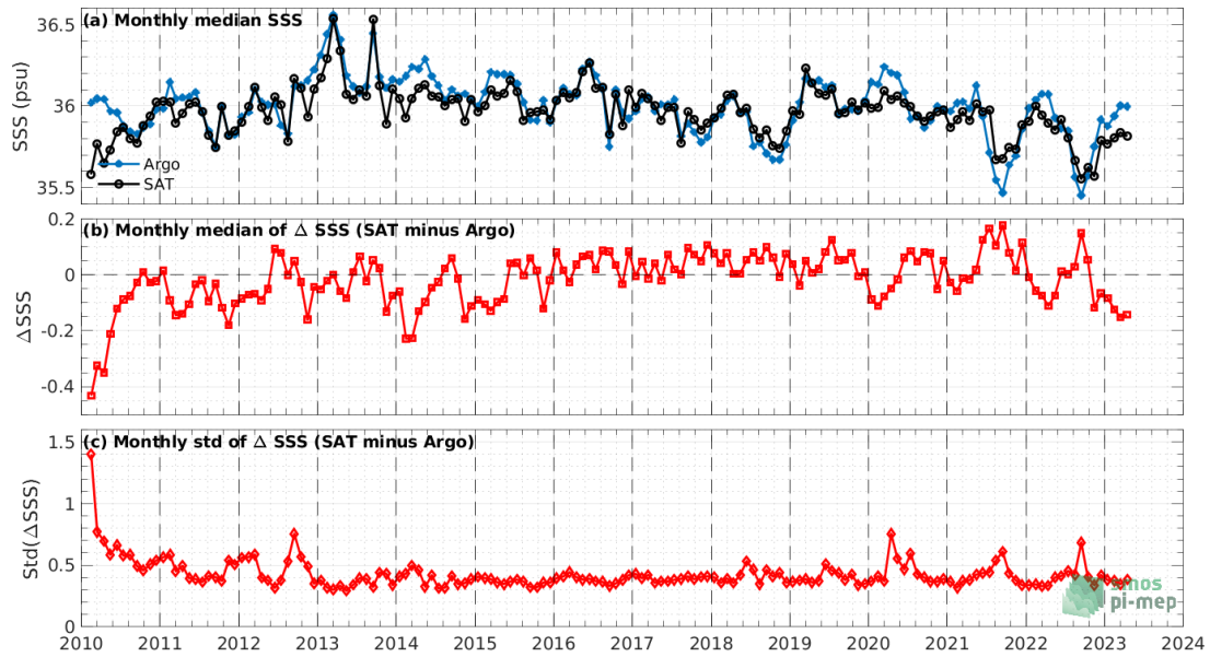
Figure 7: Time series of the monthly median SSS (top), median of \Delta SSS (Satellite - Argo) and Std of \Delta SSS (Satellite - Argo) over the North Atlantic Ocean Pi-MEP region considering all match-ups collected by the Pi-MEP.
