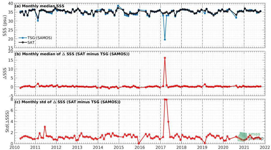
Figure 7: Time series of the monthly median SSS (top), median of \Delta SSS (Satellite - TSG (SAMOS)) and Std of \Delta SSS (Satellite - TSG (SAMOS)) over the North Atlantic Ocean Pi-MEP region considering all match-ups collected by the Pi-MEP.
