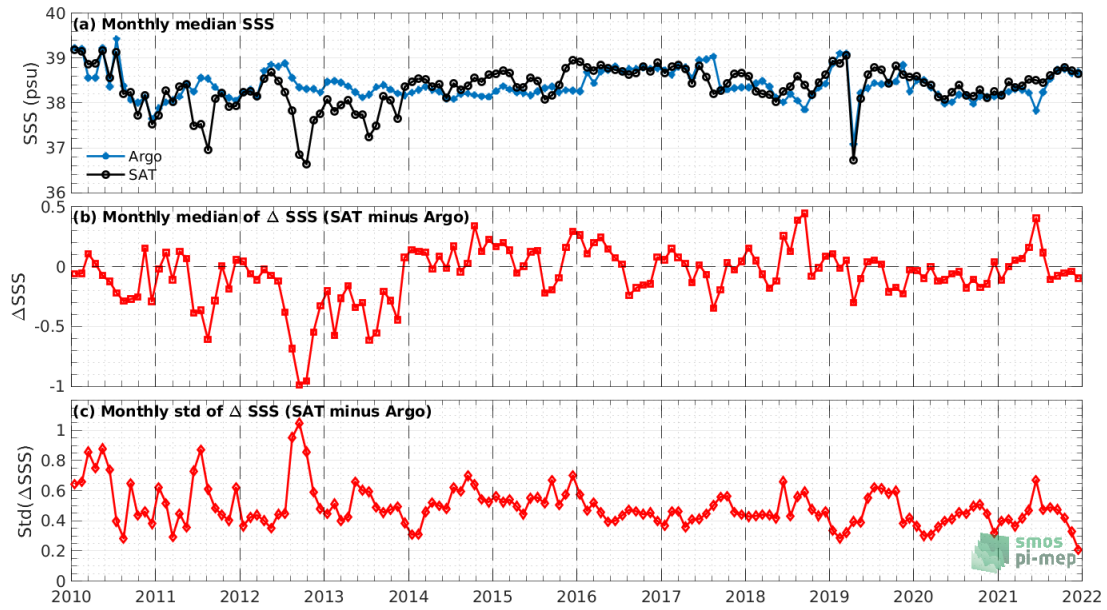
Figure 7: Time series of the monthly median SSS (top), median of \Delta SSS (Satellite - Argo) and Std of \Delta SSS (Satellite - Argo) over the Mediterranean Sea Pi-MEP region considering all match-ups collected by the Pi-MEP.
