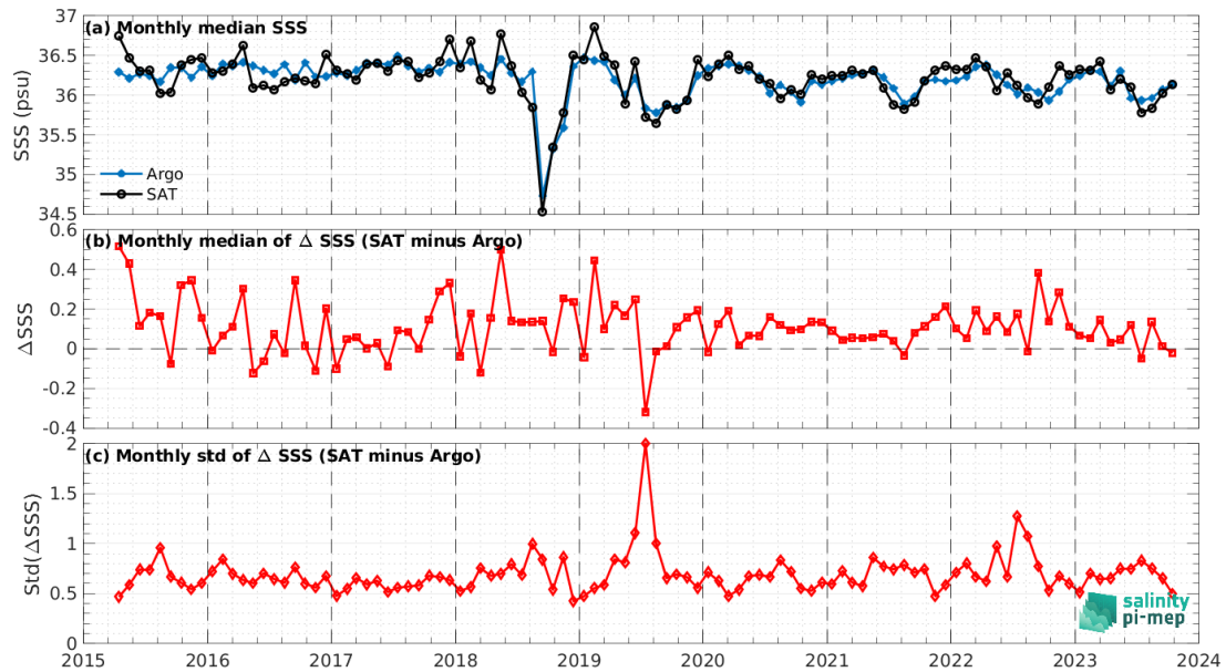
Figure 7: Time series of the monthly median SSS (top), median of \Delta SSS (Satellite - Argo) and Std of \Delta SSS (Satellite - Argo) over the Mississippi river plume Pi-MEP region considering all match-ups collected by the Pi-MEP.
