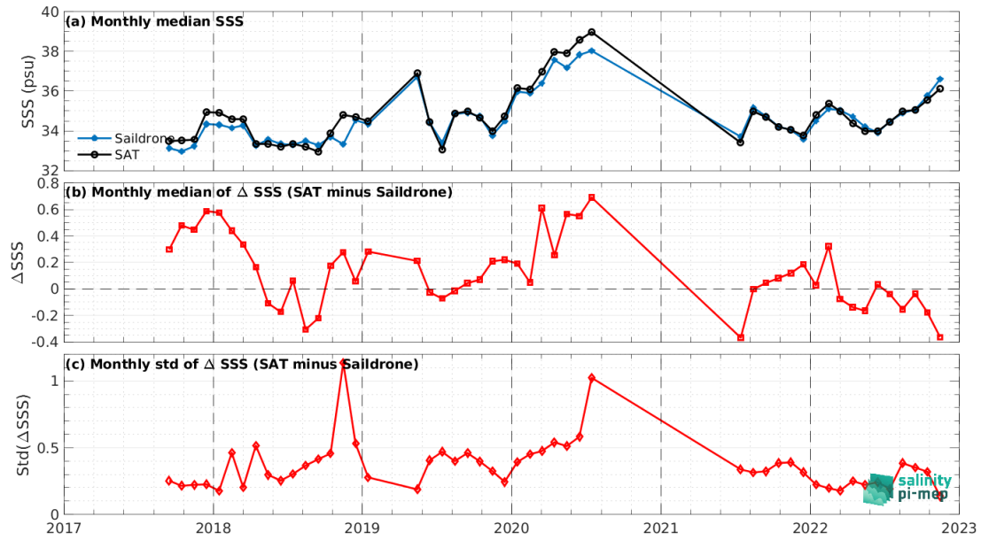
Figure 7: Time series of the monthly median SSS (top), median of \Delta SSS (Satellite - SAILDRONE) and Std of \Delta SSS (Satellite - SAILDRONE) over the Mid-Low Latitudes 45N-45S Pi-MEP region considering all match-ups collected by the Pi-MEP.
