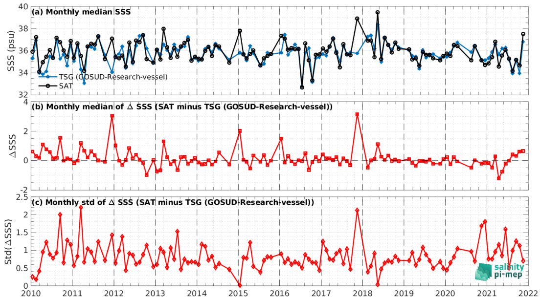
Figure 7: Time series of the monthly median SSS (top), median of \Delta SSS (Satellite - TSG (GOSUD-Research-vessel)) and Std of \Delta SSS (Satellite - TSG (GOSUD-Research-vessel)) over the Mid-Low Latitudes 45N-45S Pi-MEP region considering all match-ups collected by the Pi-MEP.
