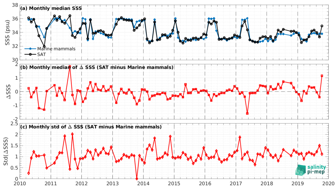
Figure 7: Time series of the monthly median SSS (top), median of \Delta SSS (Satellite - Marine mammals) and Std of \Delta SSS (Satellite - Marine mammals) over the Mid-Low Latitudes 45N-45S Pi-MEP region considering all match-ups collected by the Pi-MEP.
