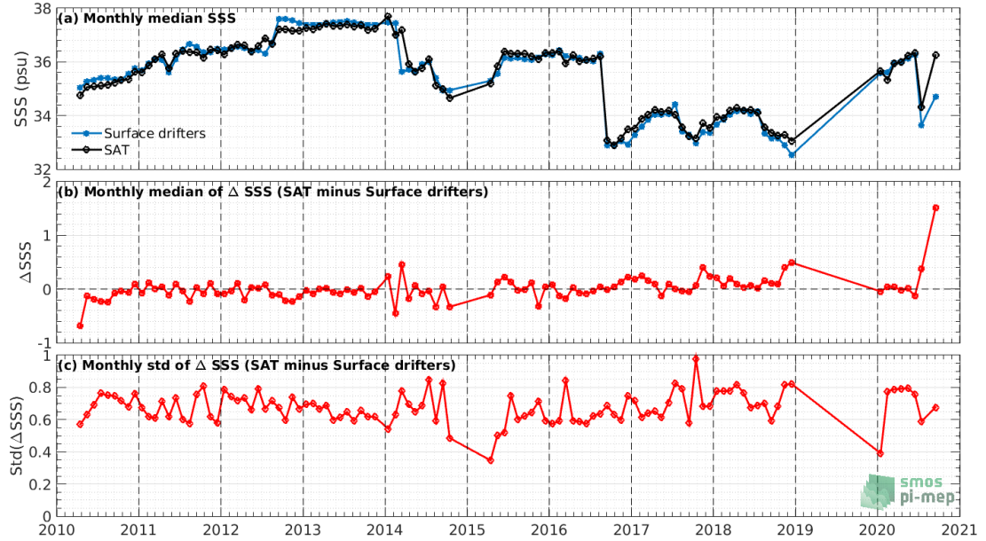
Figure 6: Time series of the monthly median SSS (top), median of \Delta SSS (Satellite - Surface drifters) and Std of \Delta SSS (Satellite - Surface drifters) over the Mid-Low Latitudes 45N-45S Pi-MEP region considering all match-ups collected by the Pi-MEP.
