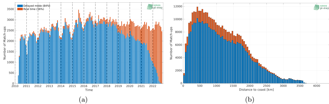
Figure 1: Number of match-ups between Argo and SMOS SSS L2 v700 (ESA) SSS as a function of time (a) and as function of the distance to coast (b) over the Mid-Low Latitudes 45N-45S Pi-MEP region and for the full satellite product period.
