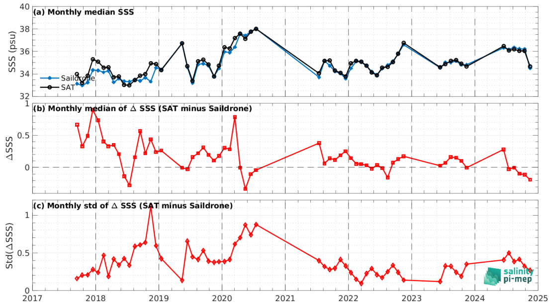
Figure 8: Time series of the monthly median SSS (top), median of \Delta SSS (Satellite - Saildrone) and Std of \Delta SSS (Satellite - Saildrone) over the Mid-Low Latitudes 45N-45S Pi-MEP region considering all match-ups collected by the Pi-MEP.
