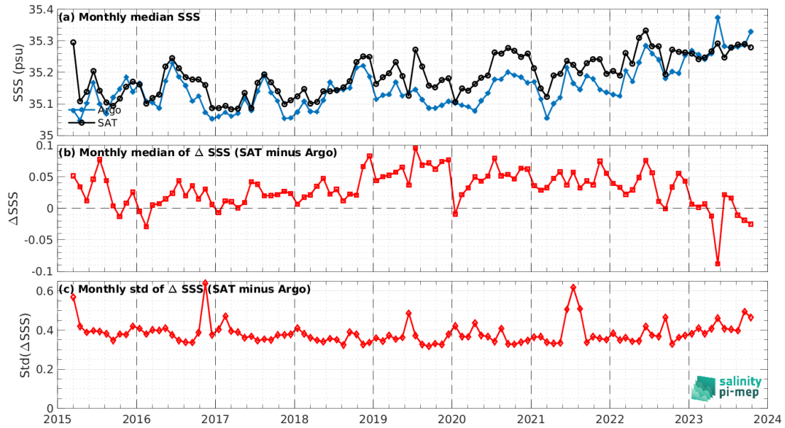
Figure 7: Time series of the monthly median SSS (top), median of \Delta SSS (Satellite - Argo) and Std of \Delta SSS (Satellite - Argo) over the Mid-Low Latitudes 45N-45S Pi-MEP region considering all match-ups collected by the Pi-MEP.
