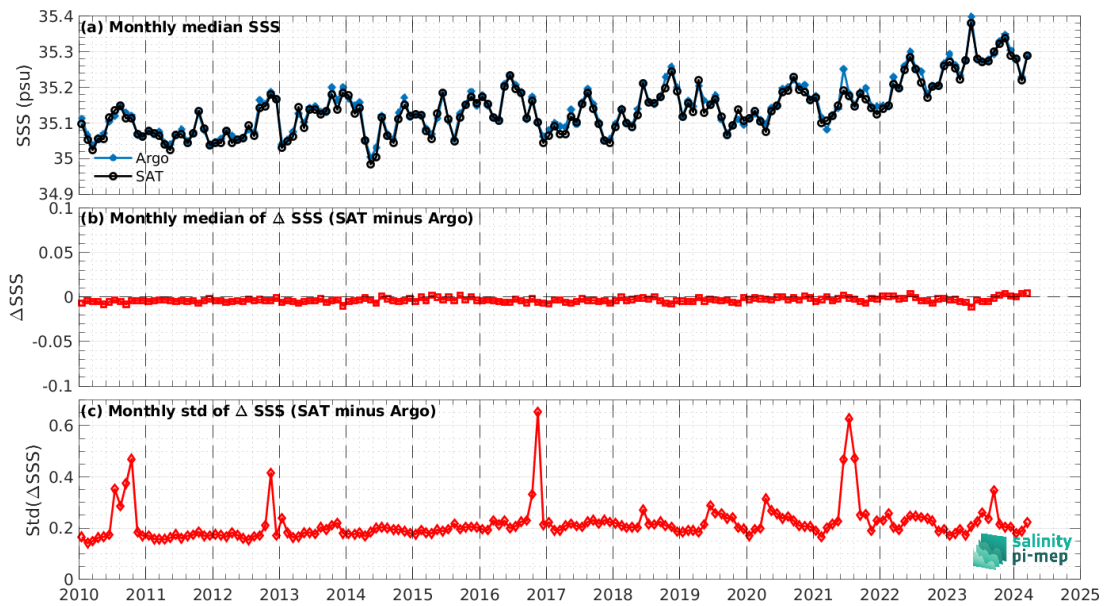
Figure 8: Time series of the monthly median SSS (top), median of \Delta SSS (Satellite - Argo) and Std of \Delta SSS (Satellite - Argo) over the Mid-Low Latitudes 45N-45S Pi-MEP region considering all match-ups collected by the Pi-MEP.
