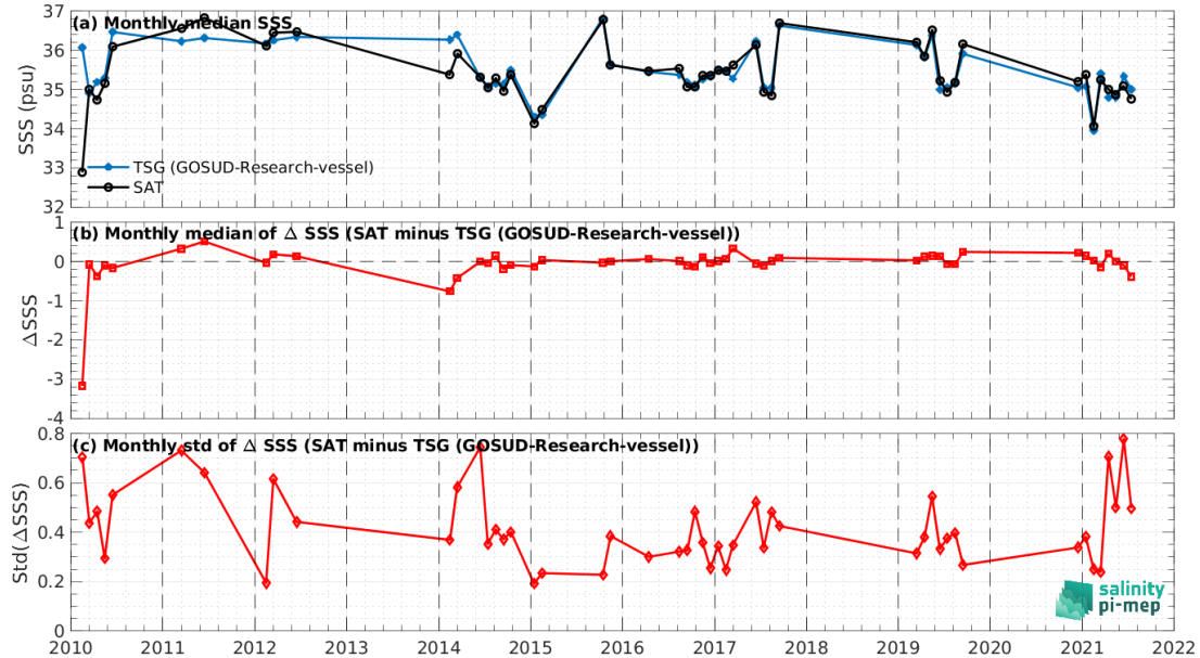
Figure 8: Time series of the monthly median SSS (top), median of \Delta\text{SSS} (Satellite - TSG (GOSUD-Research-vessel)) and Std of \Delta\text{SSS} (Satellite - TSG (GOSUD-Research-vessel)) over the Indian Ocean Pi-MEP region considering all match-ups collected by the Pi-MEP.
