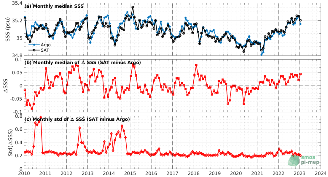
Figure 7: Time series of the monthly median SSS (top), median of \Delta SSS (Satellite - Argo) and Std of \Delta SSS (Satellite - Argo) over the Indian Ocean Pi-MEP region considering all match-ups collected by the Pi-MEP.
