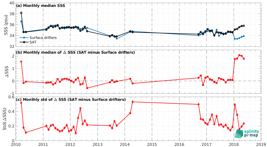
Figure 7: Time series of the monthly median SSS (top), median of \Delta\text{SSS} (Satellite - Surface drifters) and Std of \Delta\text{SSS} (Satellite - Surface drifters) over the Indian Ocean Pi-MEP region considering all match-ups collected by the Pi-MEP.
