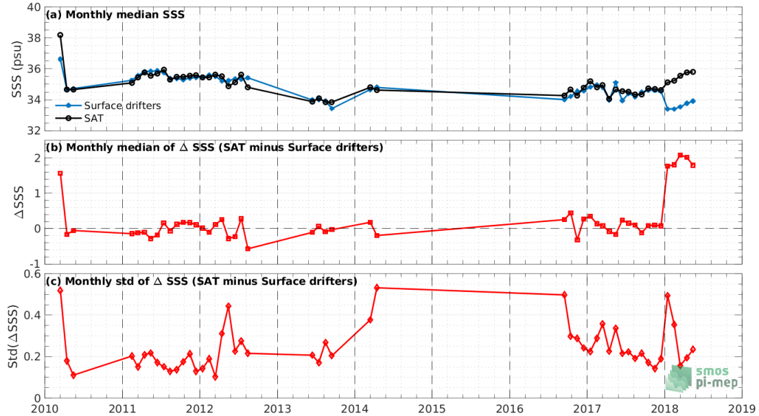
Figure 6: Time series of the monthly median SSS (top), median of \Delta\text{SSS} (Satellite - Surface drifters) and Std of \Delta\text{SSS} (Satellite - Surface drifters) over the Indian Ocean Pi-MEP region considering all match-ups collected by the Pi-MEP.
