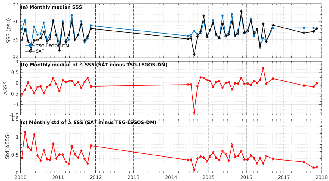
Figure 7: Time series of the monthly median SSS (top), median of \Delta SSS (Satellite - TSG-LEGOS-DM) and Std of \Delta SSS (Satellite - TSG-LEGOS-DM) over the Indian Ocean Pi-MEP region considering all match-ups collected by the Pi-MEP.
