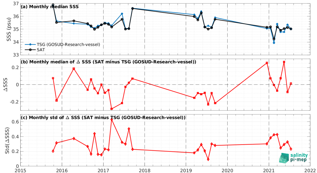
Figure 8: Time series of the monthly median SSS (top), median of \Delta SSS (Satellite - TSG (GOSUD-Research-vessel)) and Std of \Delta SSS (Satellite - TSG (GOSUD-Research-vessel)) over the Indian Ocean Pi-MEP region considering all match-ups collected by the Pi-MEP.
