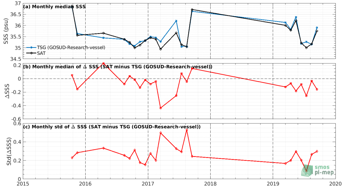
Figure 7: Time series of the monthly median SSS (top), median of \Delta\text{SSS} (Satellite - TSG (GOSUD-Research-vessel)) and Std of \Delta\text{SSS} (Satellite - TSG (GOSUD-Research-vessel)) over the Indian Ocean Pi-MEP region considering all match-ups collected by the Pi-MEP.
