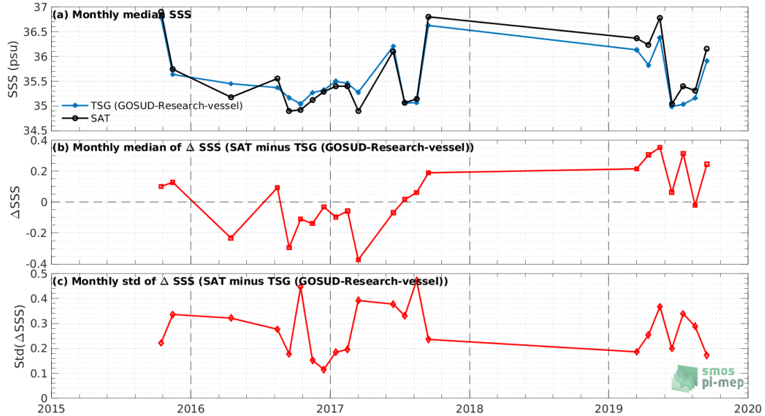
Figure 7: Time series of the monthly median SSS (top), median of \Delta SSS (Satellite - TSG (GOSUD-Research-vessel)) and Std of \Delta SSS (Satellite - TSG (GOSUD-Research-vessel)) over the Indian Ocean Pi-MEP region considering all match-ups collected by the Pi-MEP.
