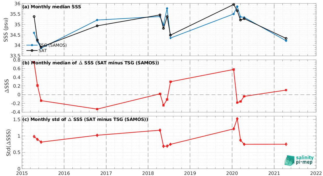
Figure 7: Time series of the monthly median SSS (top), median of \Delta SSS (Satellite - TSG (SAMOS)) and Std of \Delta SSS (Satellite - TSG (SAMOS)) over the Indian Ocean Pi-MEP region considering all match-ups collected by the Pi-MEP.
