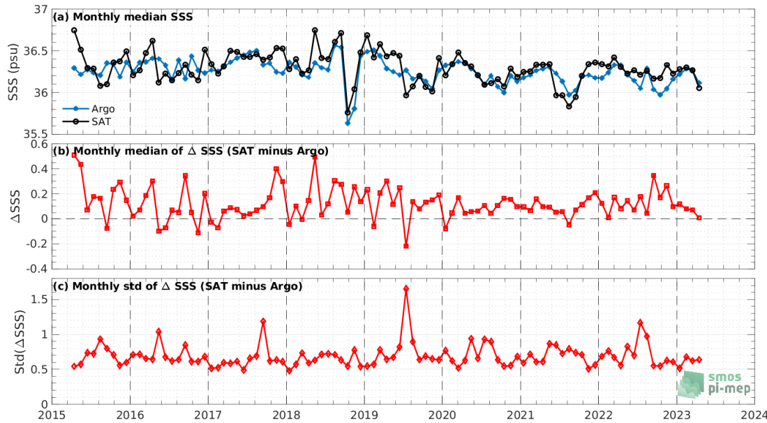
Figure 7: Time series of the monthly median SSS (top), median of \Delta SSS (Satellite - Argo) and Std of \Delta SSS (Satellite - Argo) over the Gulf of Mexico Pi-MEP region considering all match-ups collected by the Pi-MEP.
