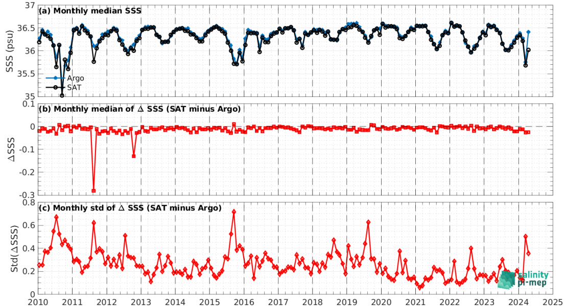
Figure 8: Time series of the monthly median SSS (top), median of \Delta\text{SSS} (Satellite - Argo) and Std of \Delta\text{SSS} (Satellite - Argo) over the Gulf Stream Pi-MEP region considering all match-ups collected by the Pi-MEP.
