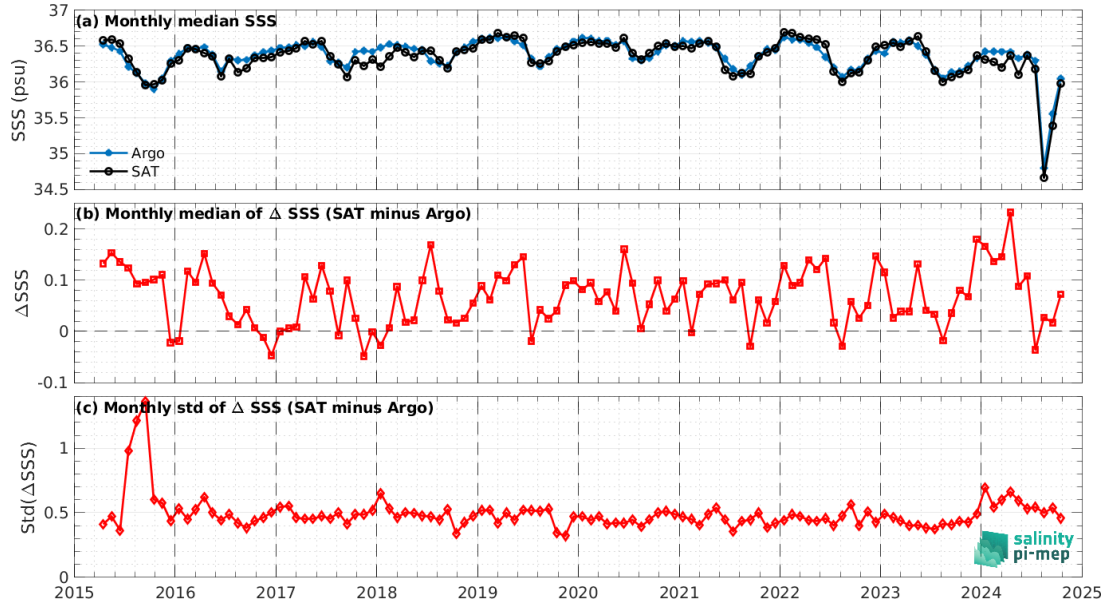
Figure 8: Time series of the monthly median SSS (top), median of \Delta SSS (Satellite - Argo) and Std of \Delta SSS (Satellite - Argo) over the Gulf Stream Pi-MEP region considering all match-ups collected by the Pi-MEP.
