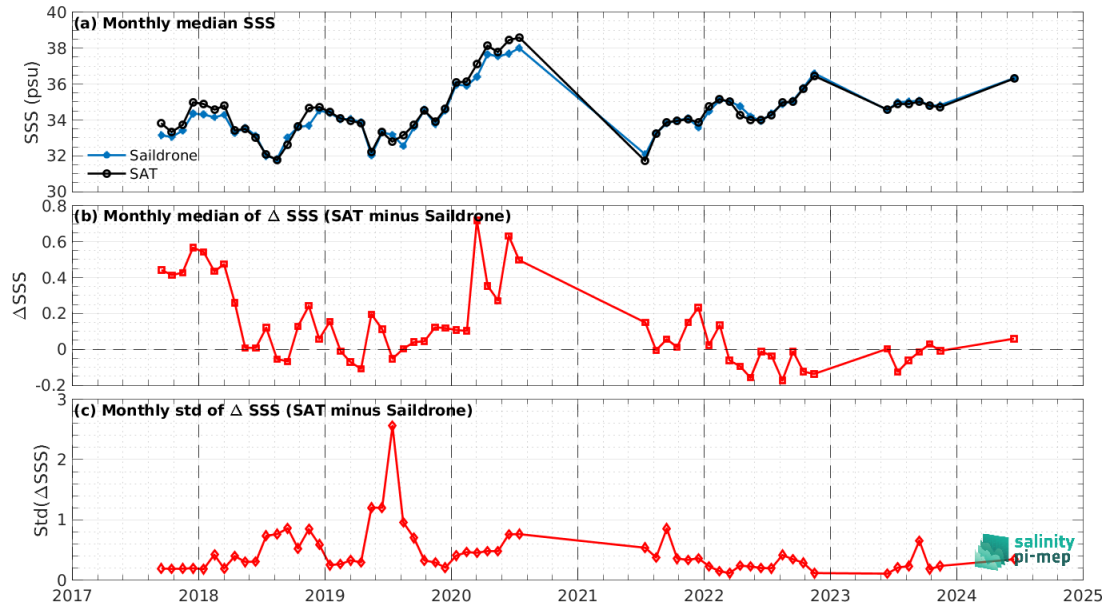
Figure 8: Time series of the monthly median SSS (top), median of \Delta SSS (Satellite - Saildrone) and Std of \Delta SSS (Satellite - Saildrone) over the Global Ocean Pi-MEP region considering all match-ups collected by the Pi-MEP.
