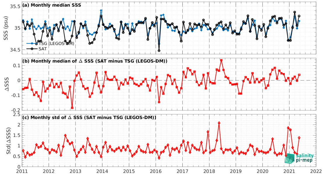
Figure 8: Time series of the monthly median SSS (top), median of \Delta\text{SSS} (Satellite - TSG (LEGOS-DM)) and Std of \Delta\text{SSS} (Satellite - TSG (LEGOS-DM)) over the Global Ocean Pi-MEP region considering all match-ups collected by the Pi-MEP.
