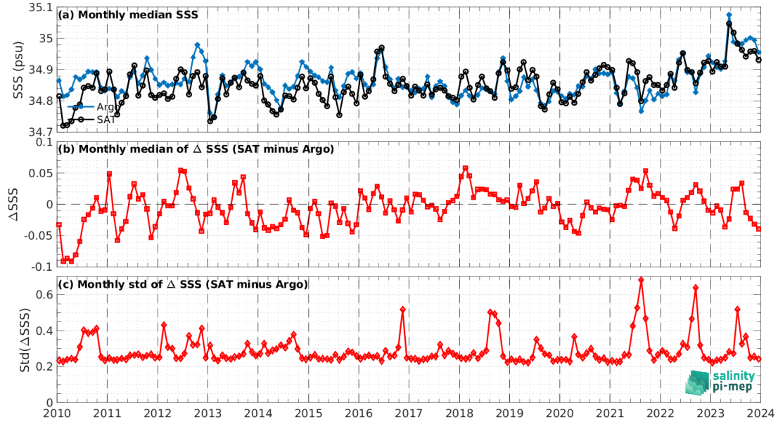
Figure 8: Time series of the monthly median SSS (top), median of \Delta SSS (Satellite - Argo) and Std of \Delta SSS (Satellite - Argo) over the Global Ocean Pi-MEP region considering all match-ups collected by the Pi-MEP.
