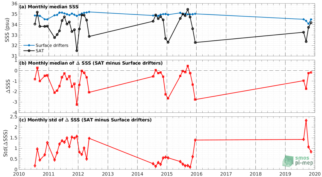
Figure 6: Time series of the monthly median SSS (top), median of \Delta SSS (Satellite - Surface drifters) and Std of \Delta SSS (Satellite - Surface drifters) over the Global Ocean Pi-MEP region considering all match-ups collected by the Pi-MEP.
