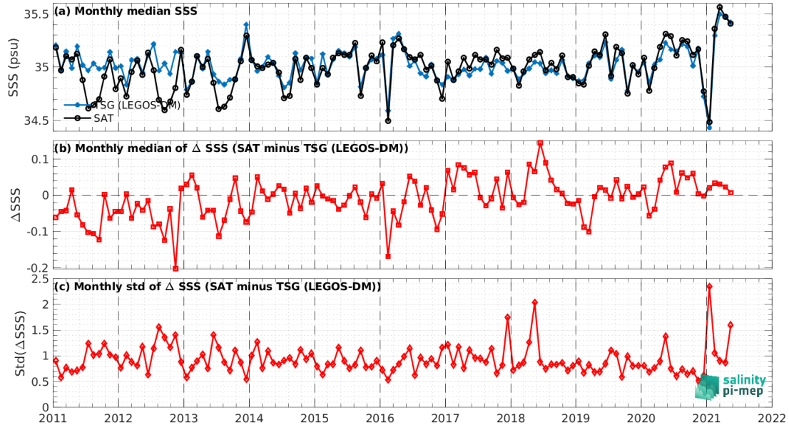
Figure 7: Time series of the monthly median SSS (top), median of \Delta SSS (Satellite - TSG (LEGOS-DM)) and Std of \Delta SSS (Satellite - TSG (LEGOS-DM)) over the Global Ocean Pi-MEP region considering all match-ups collected by the Pi-MEP.
