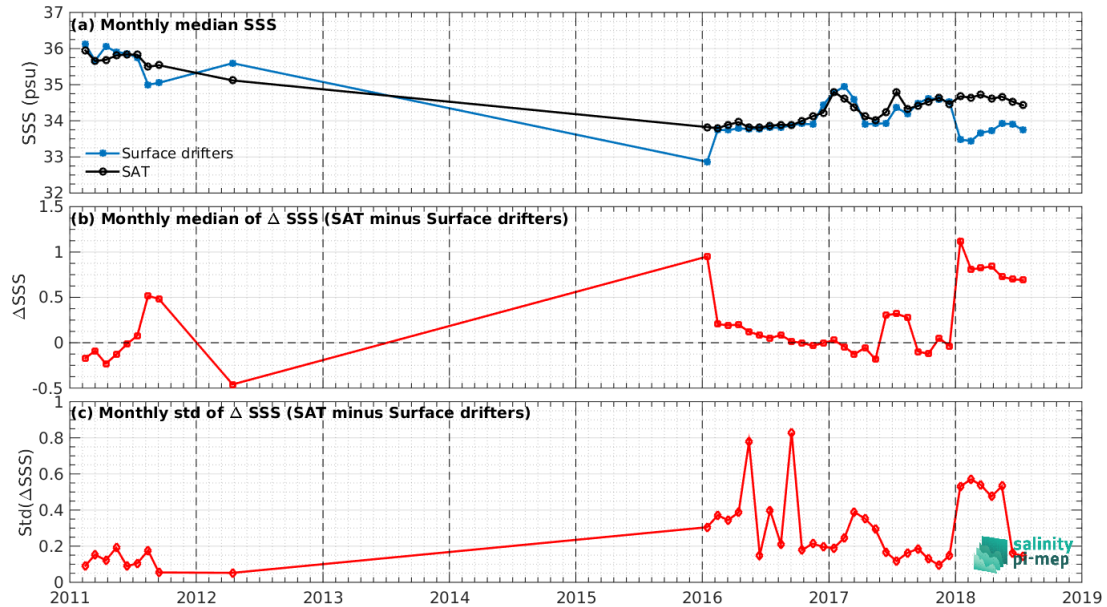
Figure 7: Time series of the monthly median SSS (top), median of \Delta SSS (Satellite - Surface drifters) and Std of \Delta SSS (Satellite - Surface drifters) over the Global Ocean Pi-MEP region considering all match-ups collected by the Pi-MEP.
