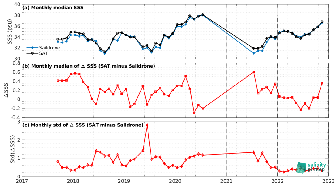
Figure 7: Time series of the monthly median SSS (top), median of \Delta SSS (Satellite - Saildrone) and Std of \Delta SSS (Satellite - Saildrone) over the Global Ocean Pi-MEP region considering all match-ups collected by the Pi-MEP.
