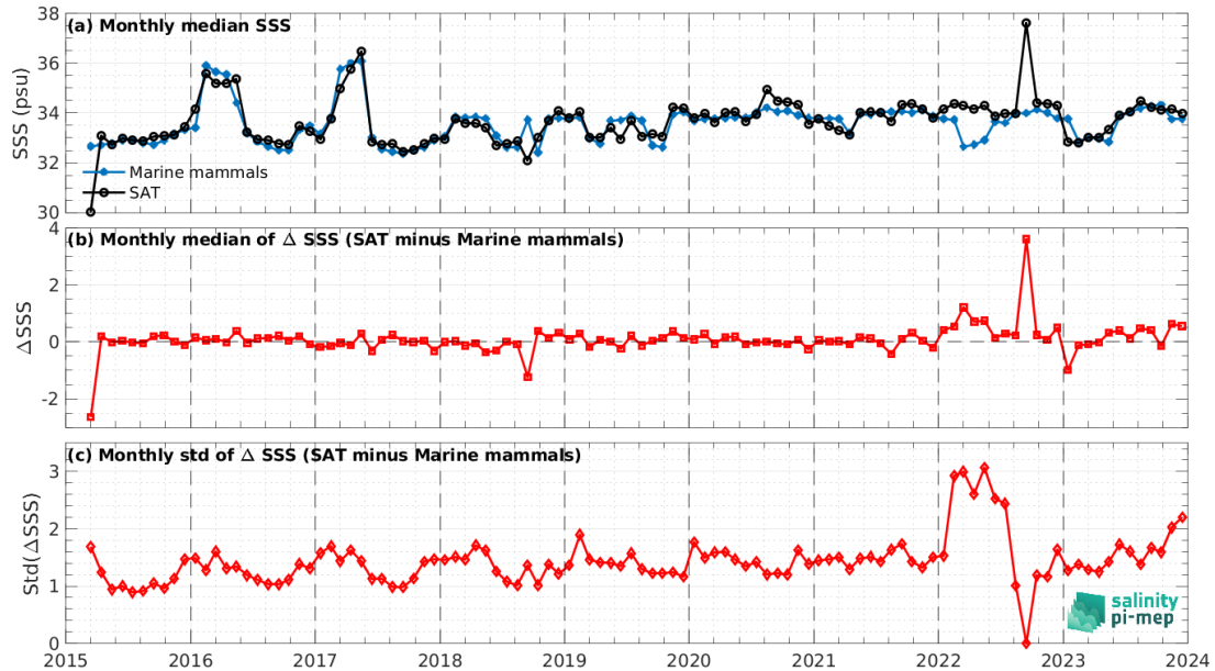
Figure 8: Time series of the monthly median SSS (top), median of \Delta SSS (Satellite - Marine mammals) and Std of \Delta SSS (Satellite - Marine mammals) over the Global Ocean Pi-MEP region considering all match-ups collected by the Pi-MEP.
