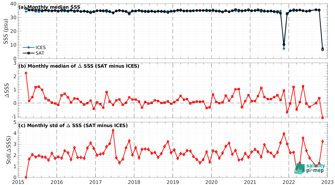
Figure 8: Time series of the monthly median SSS (top), median of \Delta SSS (Satellite - ICES) and Std of \Delta SSS (Satellite - ICES) over the Global Ocean Pi-MEP region considering all match-ups collected by the Pi-MEP.
