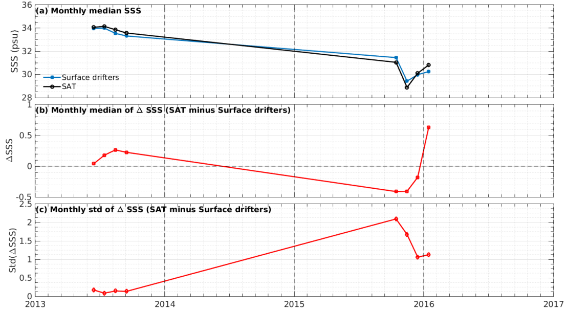
Figure 6: Time series of the monthly median SSS (top), median of \Delta SSS (Satellite - Surface drifters) and Std of \Delta SSS (Satellite - Surface drifters) over the Ganga and Brahmaputra river plumes Pi-MEP region considering all match-ups collected by the Pi-MEP.
